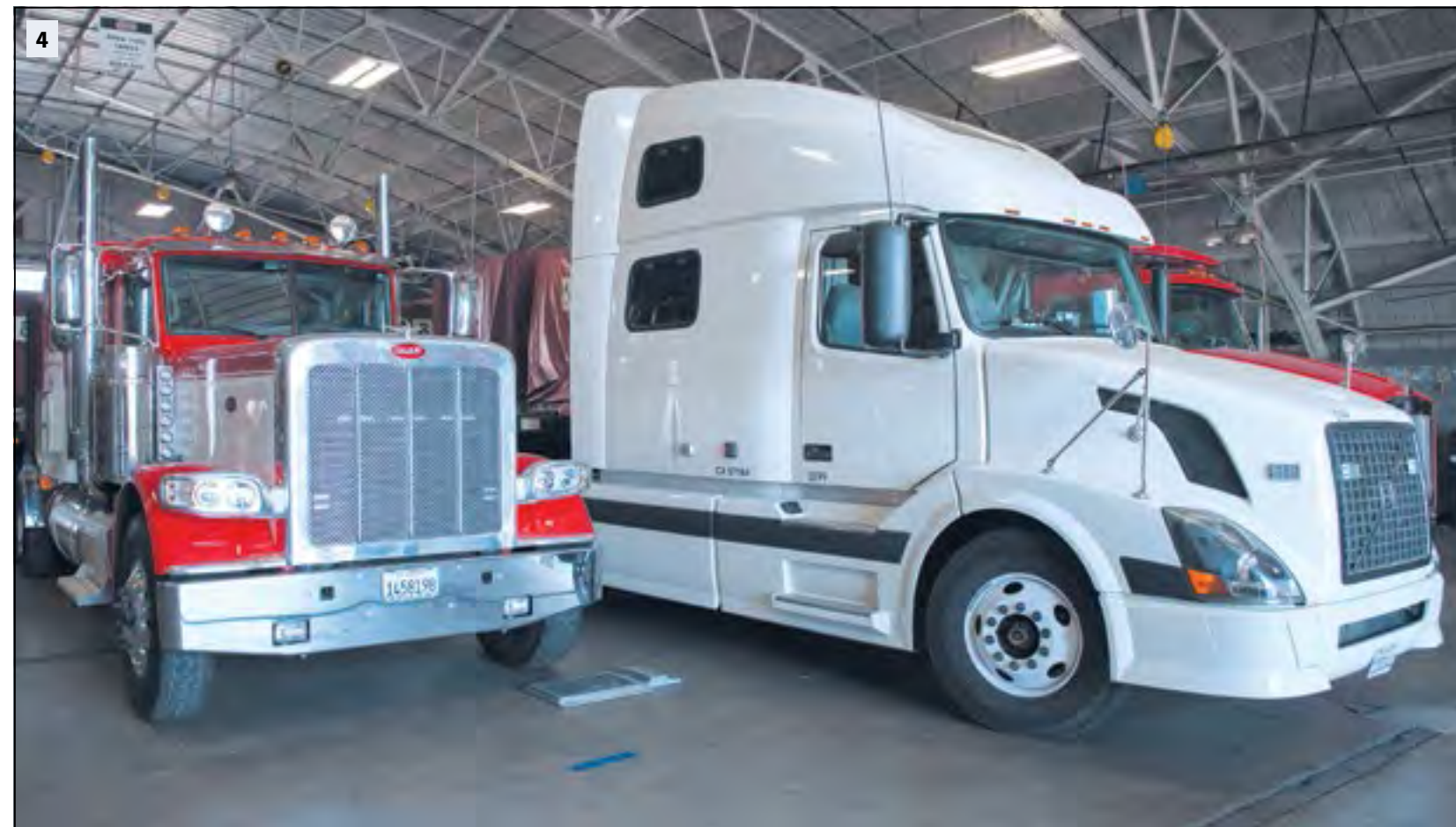
4) Cargo transport semi-trucks are used to carry equipment utilized by the California Urban Search and Rescue Task Force 7 team Aug. 23 at McClellan Park, Calif. The red truck on the left has a low profile, with removable exhaust stacks, designed to load directly onto either a C-17 Globemaster III or C-5M Super Galaxy aircraft, stationed at nearby Travis Air Force Base, Calif.
